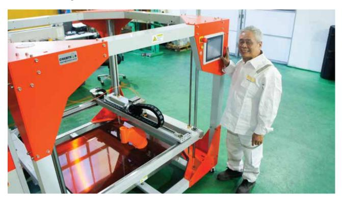
Mencast has also been busy with improving efficiency and reducing waste across all businesses. For example, we pioneered processes to 3D print propeller designs, allowing us to take advantage of process automation, dramatically reduce waste and greatly increase labour productivity.
