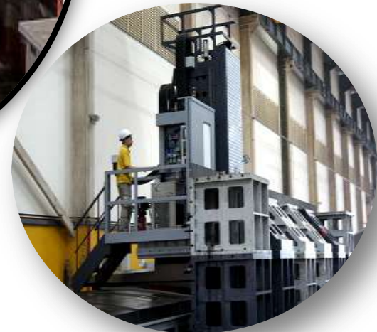
CNC Horizontal Milling Centre 20
