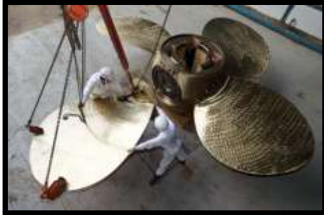
Balancing of CPP Blades and Propeller
