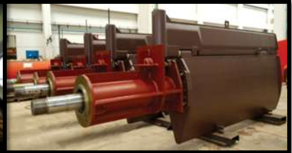
High-lift Rudder Assemblies
